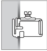
Tilt-connector, putting top lip of connector into KO, then snap downward. Insert cable, then tighten screw.
