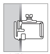
Tilt-connector, putting top lip of connector into KO, then snap downward. Insert cable, then tighten screw.
